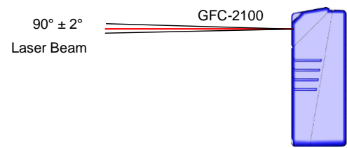
Figure 25 - GFC-2100 Laser Beam Output Position
