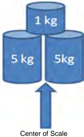
Figure 4-3 Weight Calibration Configuration for Kilograms
