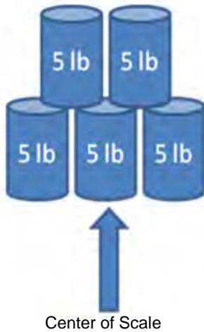
Figure 4-2 Weight Calibration Configuration for Pounds
