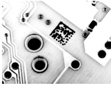
Figure 26 - Data Matrix Code Directly Marked on PCB Surface by Using Laser Etching Technology
