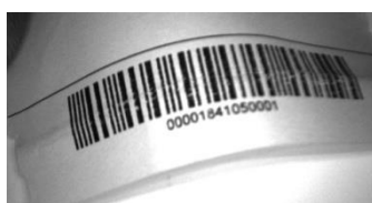
Figure 21 - Barcode Printed on Curved Surface Readable by Matrix 210N in spite of Image Optical Distortion
