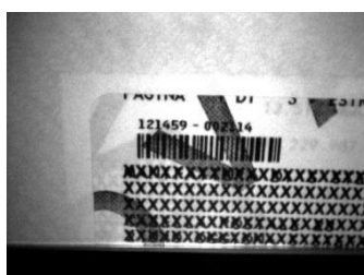
Figure 20 - Overprinted Barcode Readable by Matrix 210N also Through the Envelope Window Film
