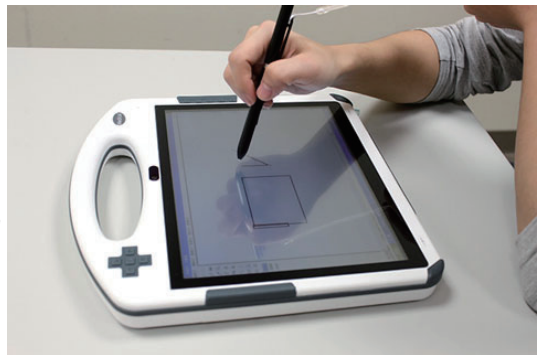
Electromagnetic digitizer with resistive touch
