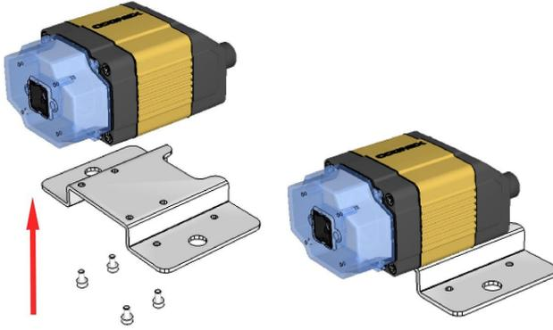
2. Mount your reader with the camera plate attached to any of the external light bracket adapters.
