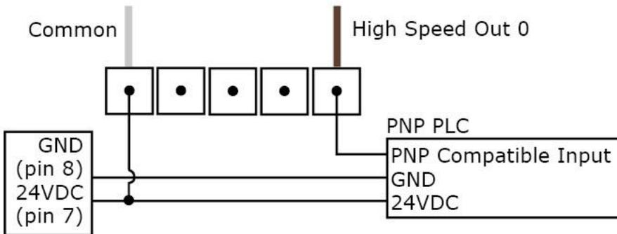
To connect the high-speed outputs to a relay, LED or similar load, connect the negative side of the load to the output and the positive side to +24V. When the output switches on, the negative side of the load is pulled down to less than 3V, and 24V appears across the load. Use a protection diode for a large inductive load, with the anode connected to the output and the cathode connected to +24V.
