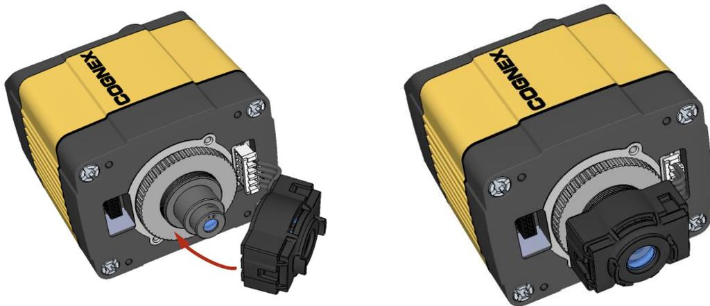
4. Place the **DM360-HPIL-RE-01** or **DM360-HPIL-RE-P-01** unit on the front of the device.
