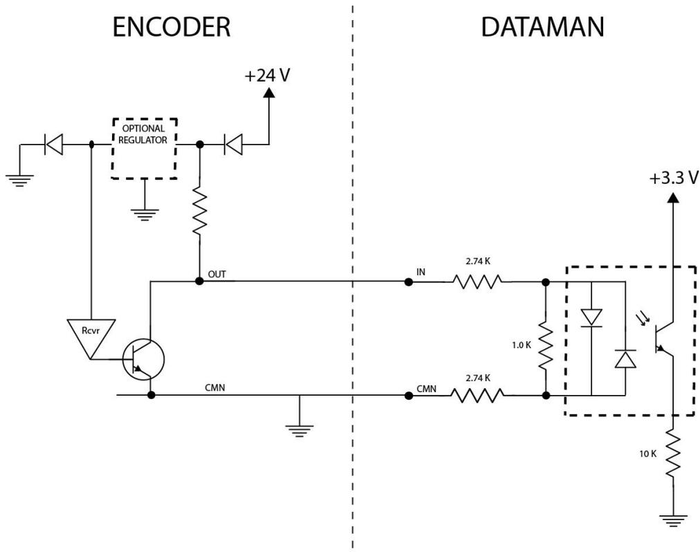
According to the speed of the line, set the number of pulses per revolution on the wheel by using the switches on the encoder (for more information, see the encoder documentation). The number of pulses, however, must not exceed 150 Hz.
