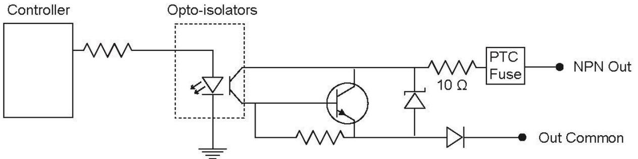
For PNP lines, the external load should be connected between the output and the negative supply voltage (0V). When connected to a 24VDC power supply, the outputs pull up greater than 21V when ON, and current flows through the load. When the outputs are OFF, no current flows through the load.
