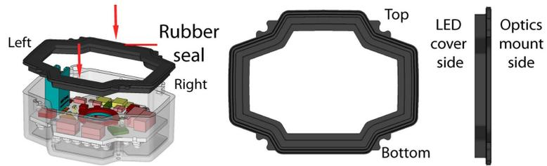
**Note:** The seal can only be installed in the correct orientation.
