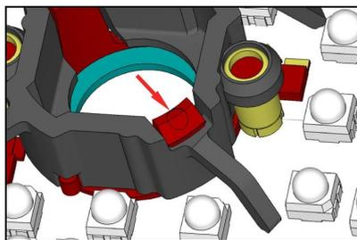
6. Insert the PCB with the filter retaining clip and the filter holder back into the front cover. Ensure that the hole in the PCB meets the orientation pin in the front cover. Fix the PCB with two Torx 6 screws of size 2.0x5 mm.
