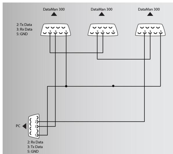
You must connect each DataMan 300 to the DataMan Setup Tool using a USB connection and set the DataMan for multi-port operation. To configure a DataMan 300 for multi-port operation, click the **Enable Multi-Port (RS-232 Sharing)** checkbox in the **Communications** application step's **Advanced** tab.
