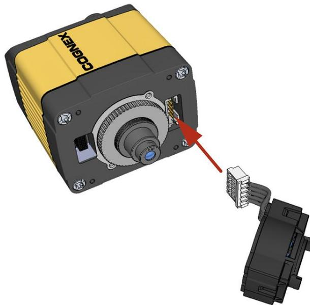
3. Attach the **Liquid Lens** to the front side of the **24mm Lens**.
