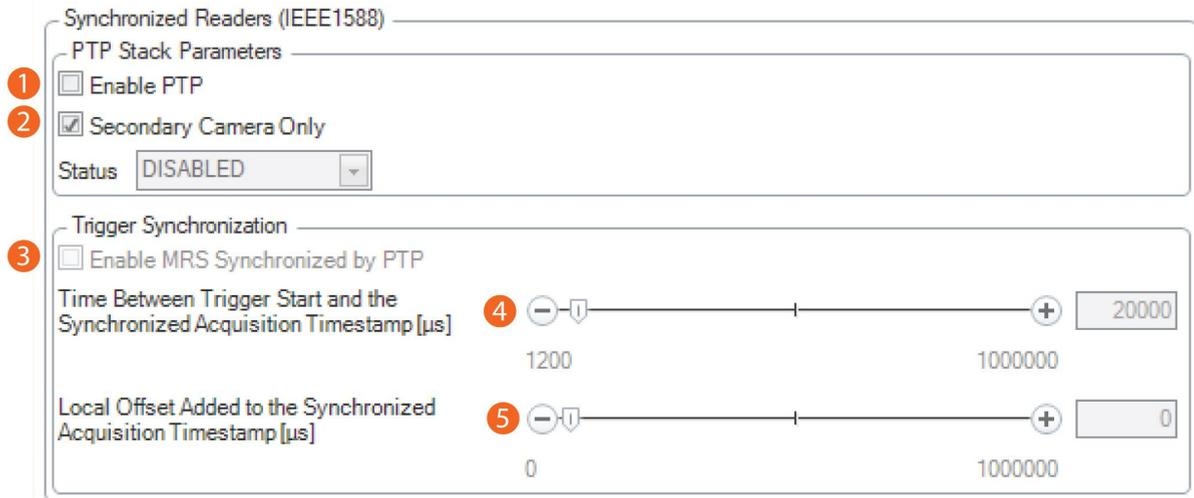
**Note:** The DataMan 300 readers use IEEE1588 for high-speed trigger synchronization.
