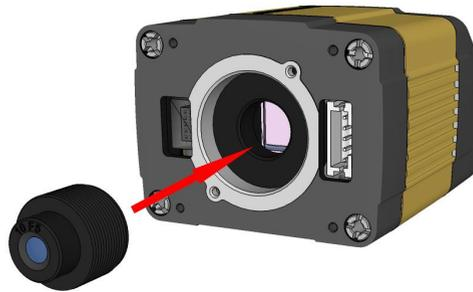
3. Press the rubber lens-locking cone into the reader. While carefully avoiding rotating the lens, press the rubber lens cone into the reader until it snaps into place around the nose of the lens.
