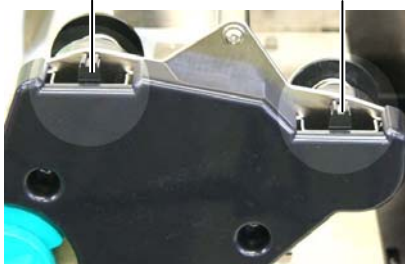
Ribbon Holder Adjustment Lever
