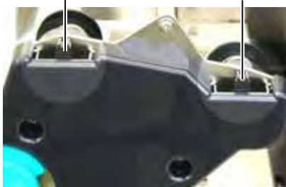
Ribbon Holder Adjustment Lever
