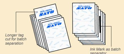
The printer separates tags by cutting the first tag longer or using the ink roller mechanism to place an ink mark on the side of each batch separator tag.
