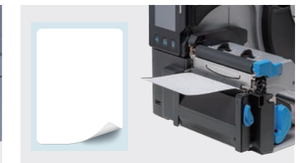
Dispenser Can either rewind the peeled liner internally or let it drop from the front of the printer.
