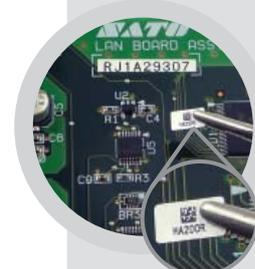
Electronic Components and Circuit Boards (PCB) Labelling
