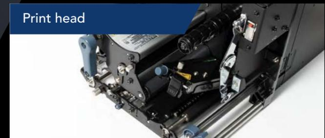
Print mechanism framed with aluminum extrusions (instead of welded plates) for added ruggedness.
